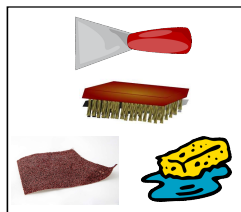
Remove loose flaking paint Wire brush rusted metal Sand, dust + clean Apply correct primers + undercoats
